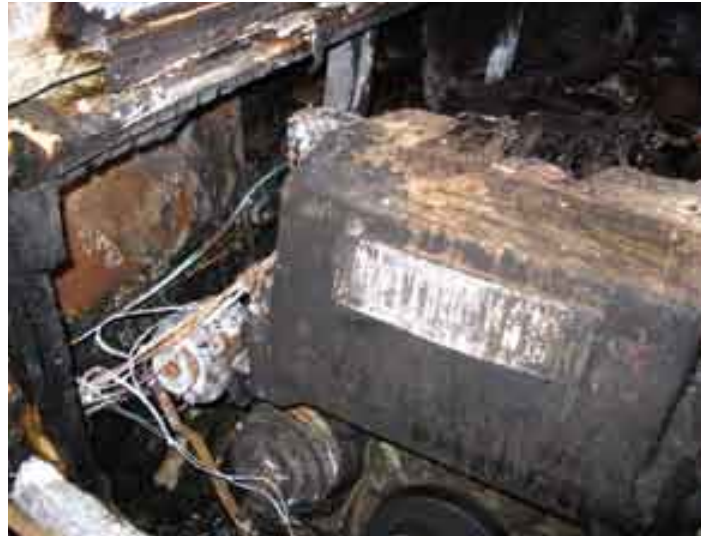
▲ THE STARBOARD ENGINE FIRE WAS "ELECTRICAL" WHEN IT BEGAN, BUT PROGRESSED INTO A GENERAL FIRE, WITH A VARIETY OF SUBSTANCES, INCLUDING FOAM RUBBER, PLASTIC, WIRE INSULATION, OIL, METAL, GREASE AND DEBRIS, WOOD AND PAINT.
