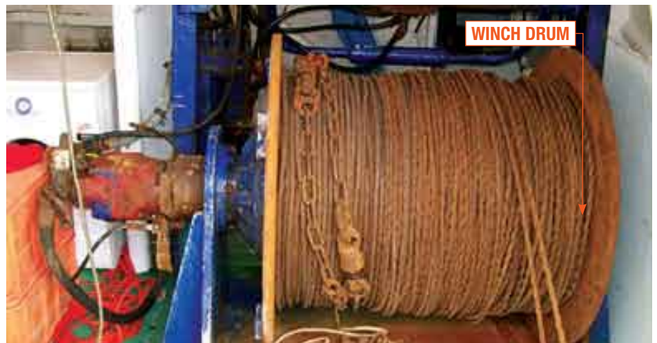
▲ THE OPERATOR MUST STAND BEHIND THE WINCH AND MONITOR THE WIRE LEVEL, AS WELL AS THE SPEED AND AMOUNT OF WIRE RETRIEVED SO FAR.
