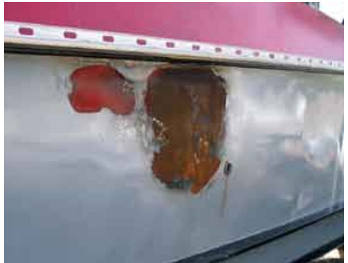
▲ A HEAVY OXIDATION PATTERN WAS VISIBLE ON THE OUTSIDE OF THE HULL AS A RESULT OF THE FIRE.
