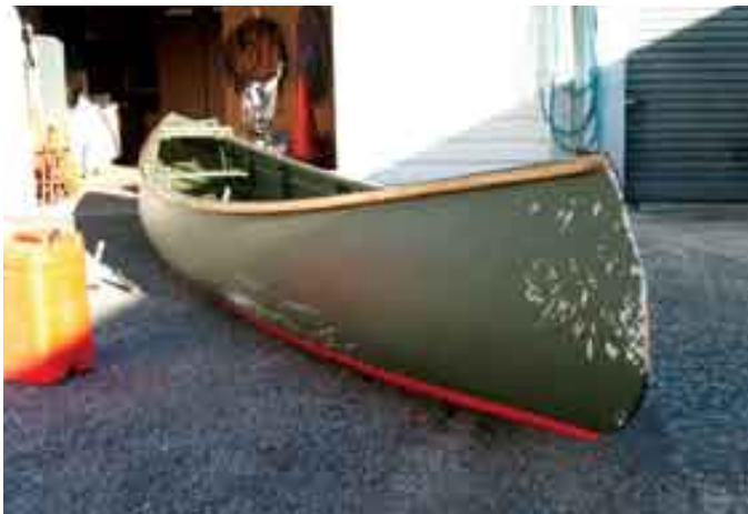
▲ CANADIAN OR OPEN-TOPPED CANOES ARE POPULAR FOR RECREATIONAL USE AND DUCK SHOOTING, AS THEY ARE CAPABLE OF CARRYING HEAVY OR BULKY LOADS AND EQUIPMENT. THEY ARE LESS RESILIENT TO THE EFFECTS OF SWAMPING THAN CLOSED-TOP KAYAKS.
