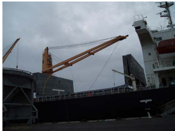
Photograph 3 – No. 4 crane after the wire parted
