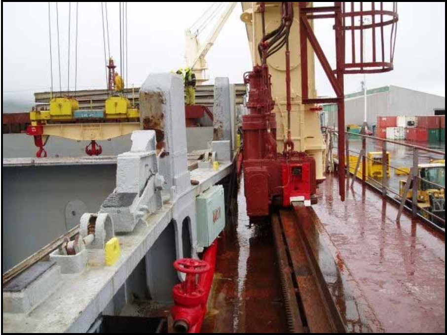
Photograph 6 View of number 5 hatch coaming from aft showing the gantry crane adjacent to the restricted space in way of the king beam
