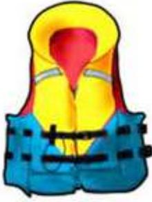
These provide at least 71 newtons of buoyancy and must have a buoyant collar to support the wearer's head. They are quite comfortable to wear continuously while boating, and are the most common PFDs found on recreational craft.
