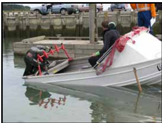
Photograph 17 Viper 1 in the stability test at 26 minutes.
