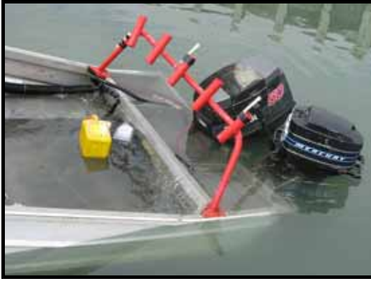
Photograph 21 Viper 1 in the stability test at 33 minutes.
