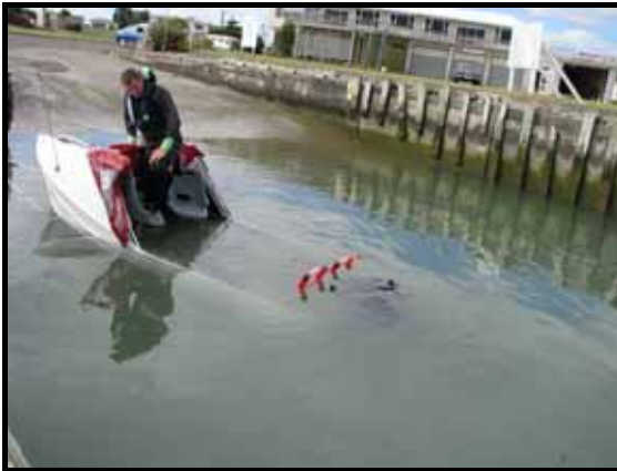
Photograph 22 Viper 1 in the stability test at 34 minutes.
